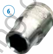
6 Degreased, since grease would destroy the protective gas atmosphere in hardening.
