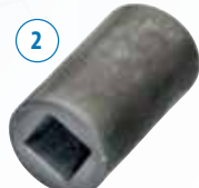
2 Hot forged in the forging press.
