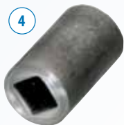
4 Outside diameter turned and knurled. For this step and the next, GEDORE uses high-tech machinery from its in-house mechanical engineering department.
